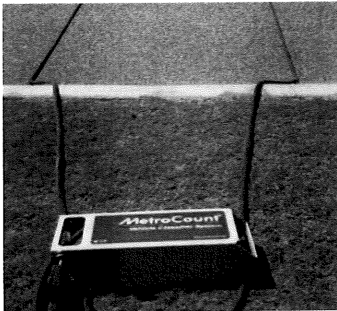
Pneumatic Tube System
